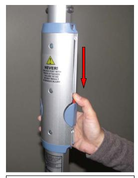
Step 3a: Press the red button down to release the safety lock.
