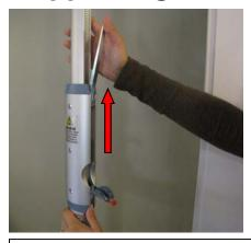
Step 7a: Push the lever up to engage with magnet.
