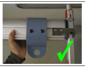
Note: Ensure track connector is sitting properly on the spring pin as shown above.
