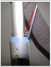
Step 7c: Make sure the bottom pin touches the plastic cover.
