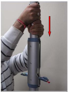
Step 4a: Grab and Push down on the top section of post with two hands as shown in Picture.
