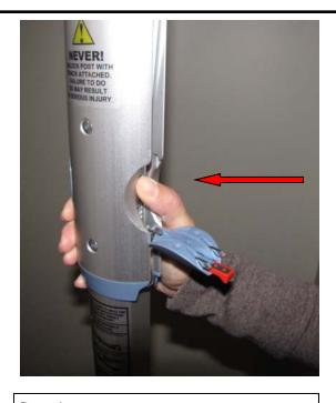
Step 4: Press the lever in all the way to release the pressure from the ratchet.
